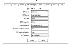
Turn On/Off SRT and set up the SRT Mode, SRT Server, SRT Port, SRT Encryption, SRT Password, SRT Bandwidth Overhead, SRT Variable Latency and SRT StreamID.
